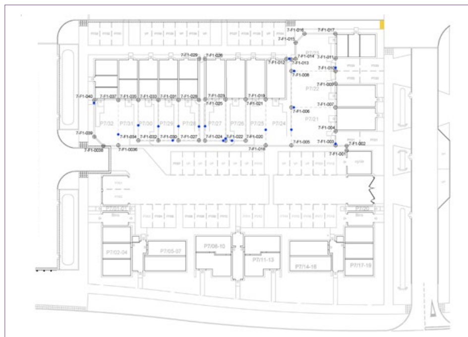
Locations for swift and bat bricks are marked onto working drawings for bricklayers
